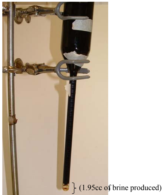
Figure 6: Imbibition Flask Showing Yates Core in Oil and Brine Produced by Spontaneous Imbibition of Yates Oil.
