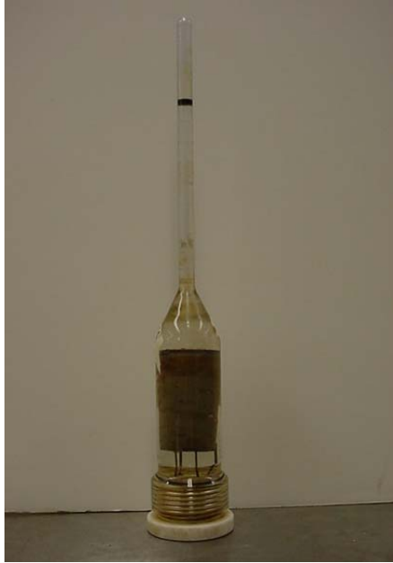
Figure 5: Imbibition Flask Showing Yates Core and Oil Produced by Spontaneous Imbibition of Yates Brine at 1500 ppm Ethoxy Alcohol Surfactant Concentration.
