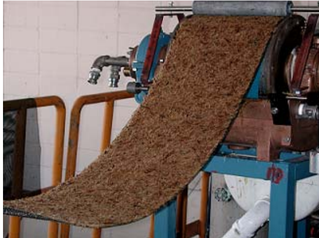
Fig. 12 – Mat detachment using a supporting plastic net
