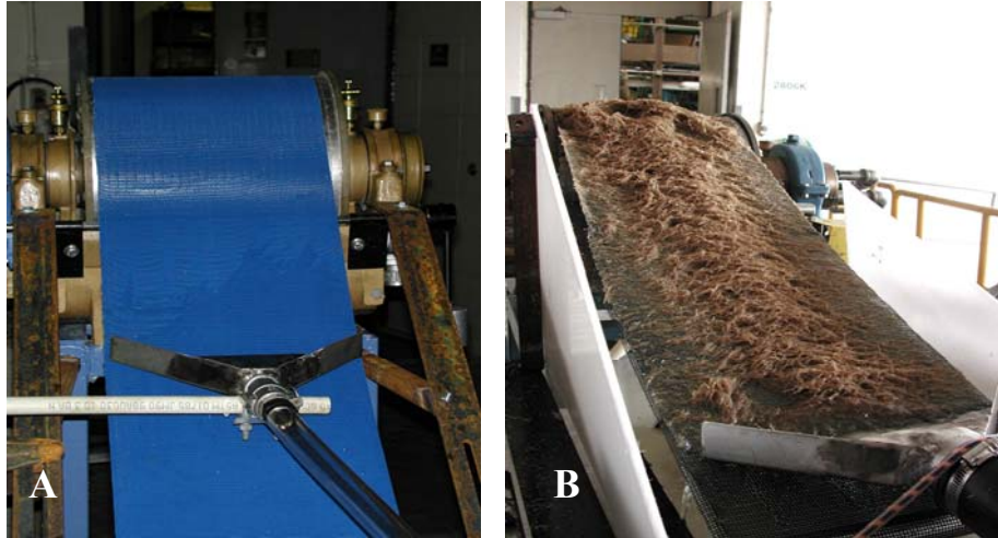
Fig. 9 – The third design (A – the nozzle; B – mat formation)
