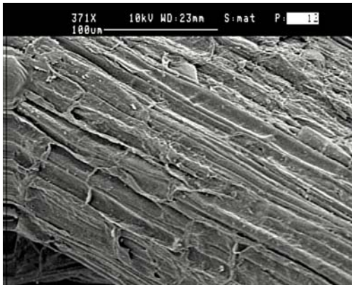
Fig. 27 – Pith cells viewed with SEM (scale 100 µm)
