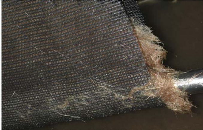
Fig. 8 – Problems in the second design (the bagasse fibers trapped inside the belt)
