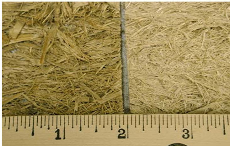
Fig. 22 – Mat comparison (on the left: original fibers, on the right: blended fibers) (scale in inches)
