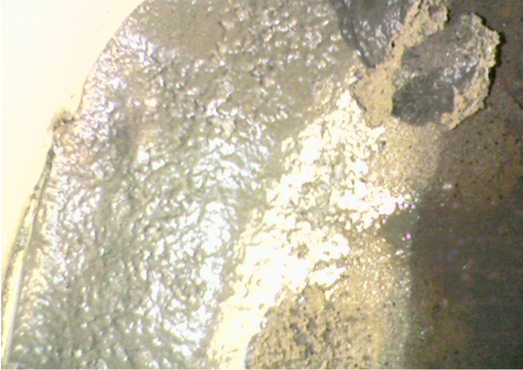
Figure G.3. SAC Column. Mud is visible on the surface of the resin.
