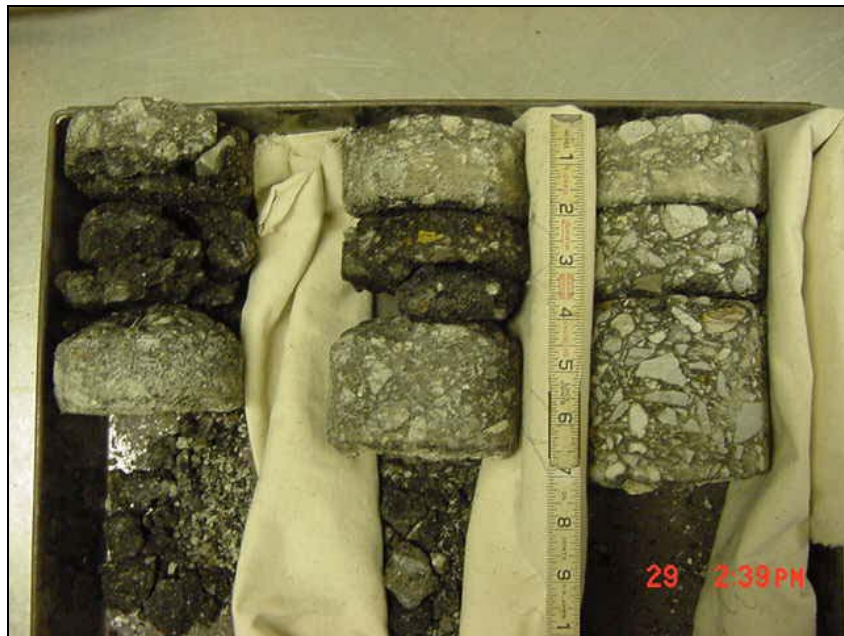
Figure 5-15. Cores taken from LA 3234 Hwy
