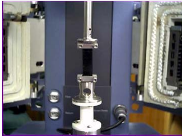
Figure 2-2. Setting of the instrument in DMA mode. ETC open
