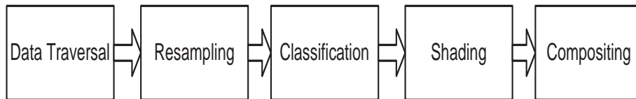
Figure 2.5: Ray casting pipeline
