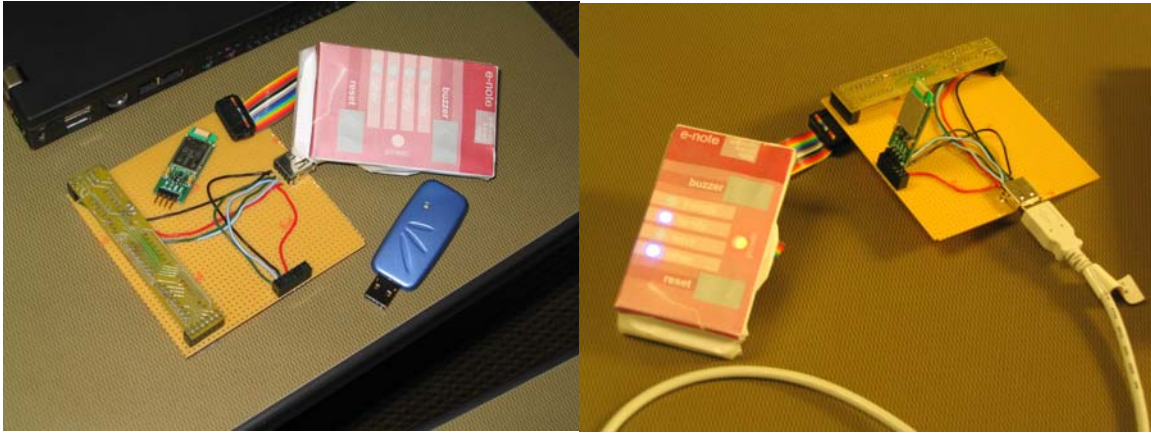
Figure [4.10] eNote individual components and when functional
