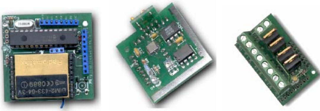
Figure [3.6]: Lancaster Mini Core, Add-on board with acceleration, light, temperature and touch sensor, Actuator Add-on board
