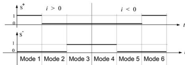
Figure 17.7. Combinations of switching signal values and the sign of output current
