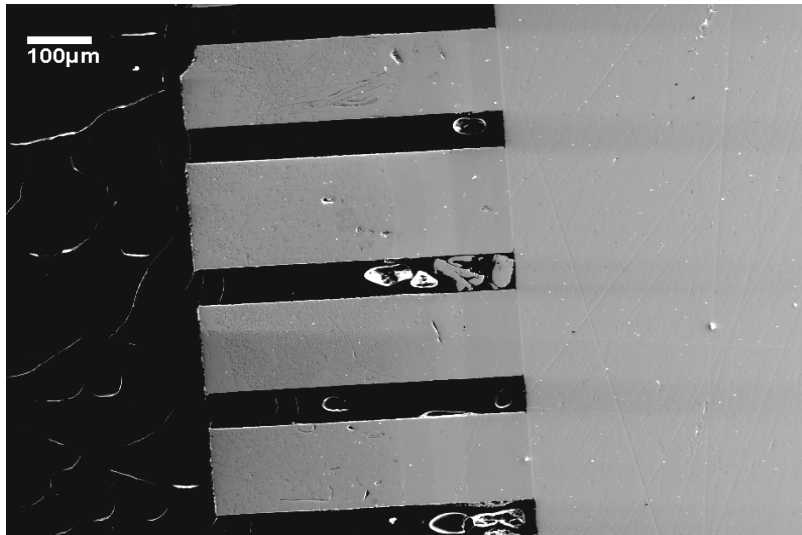
Figure 5.19: SEM micrograph of of 500 \mu\text{m} tall microposts' cross-section obtained from Bath #4 by galvanostatic step ramp pulsing with a duty cycle of 0.25.
