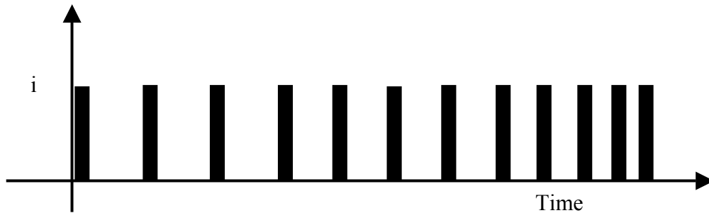
Figure 5.21: Schematic of the Pulsing Scheme showing ‘Off’ Time Reduction with Time
