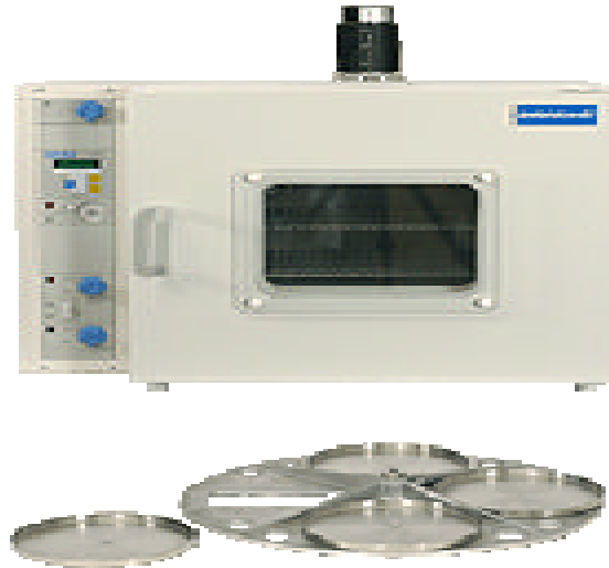
Figure 2.2.2-2 TFOT instrument (adapted from Controls Testing Equipment LTD)
