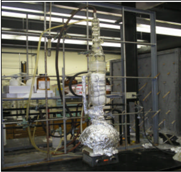
Figure 2.2.1-1 Picture of Soxhlet apparatus for extraction
