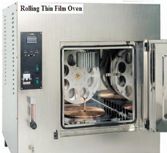
Figure 2.2.2-1 RTFOT instrument (adapted from Controls Testing Equipment LTD)
