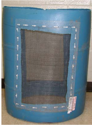
Figure 3.3. Enclosure design: window dimensions 35 cm X 51 cm, interior mesh 3 mm and exterior mesh 6.4 mm. Removal of water and nekton from within the enclosure.
