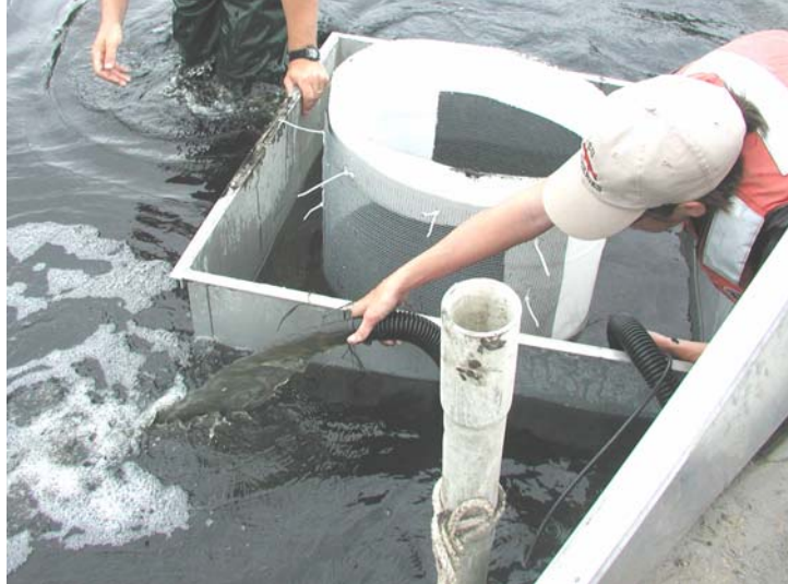
Figure 3.3. Enclosure design: window dimensions 35 cm X 51 cm, interior mesh 3 mm and exterior mesh 6.4 mm. Removal of water and nekton from within the enclosure.
