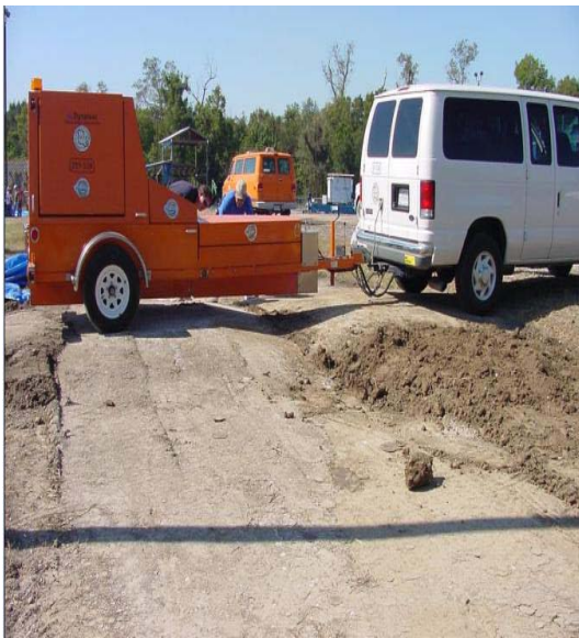
Figure 3.8 Conducting tests on cement-soil and crushed lime stone sections at ALF site
