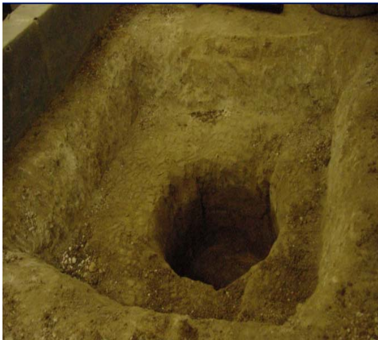
Figure 5.2 The constructed mold within soil in test box
