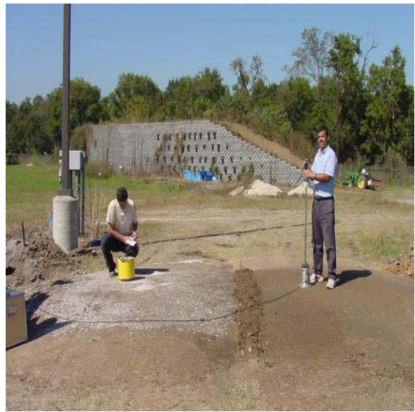
Figure 3.8 Conducting tests on cement-soil and crushed lime stone sections at ALF site
