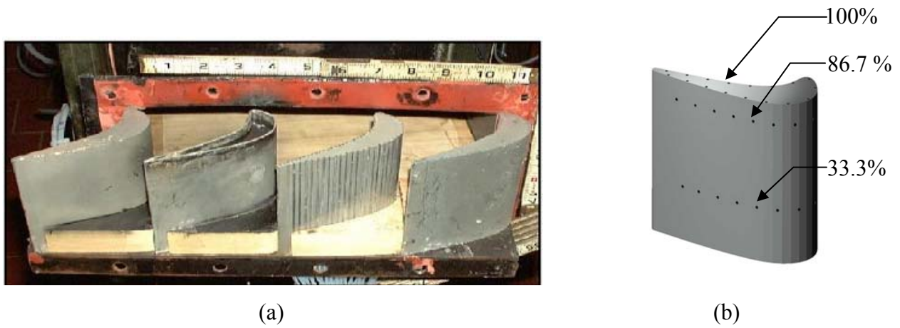
Figure 4.5: (a) Four bladed linear cascade, (b) Pressure blade
