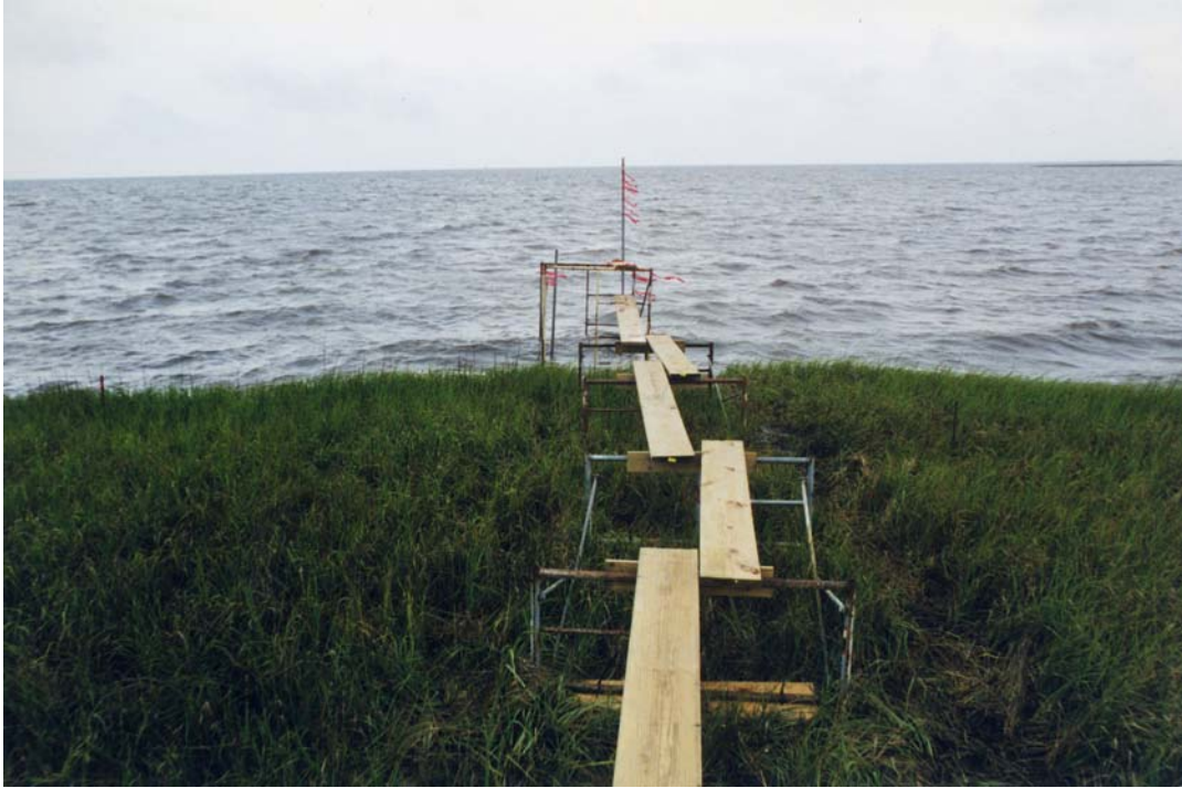
Figure 5: Hydrodynamic data were collected by submerged sensors placed at the end of the platforms on the north and south shorelines.
