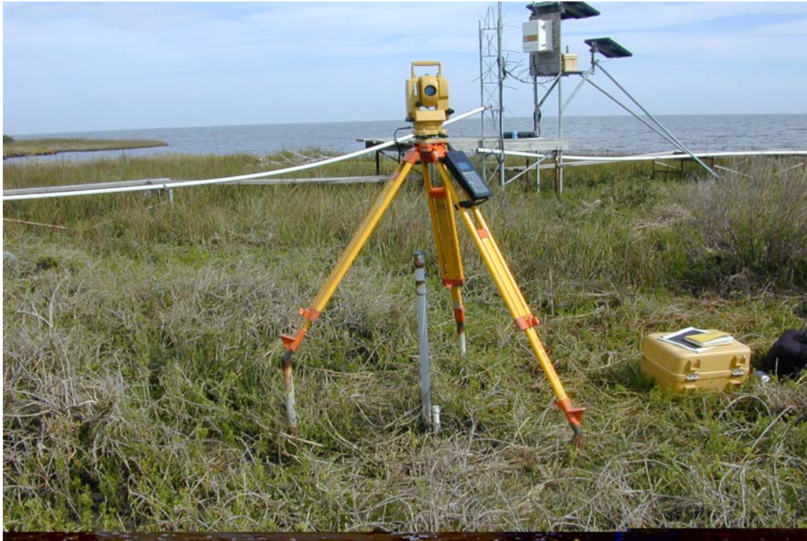
Figure 3: Topcon electronic total station and equipment used for the surveys, instrumentation in collects meteorological data.
