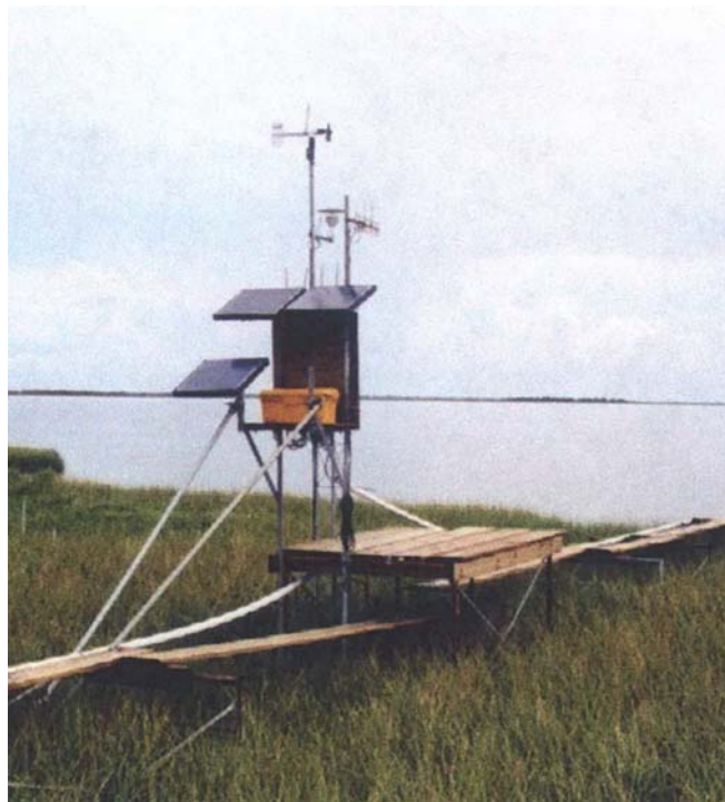
Figure 6: Meteorological instrumentation collected data from a platform constructed in the middle of the marsh island.
