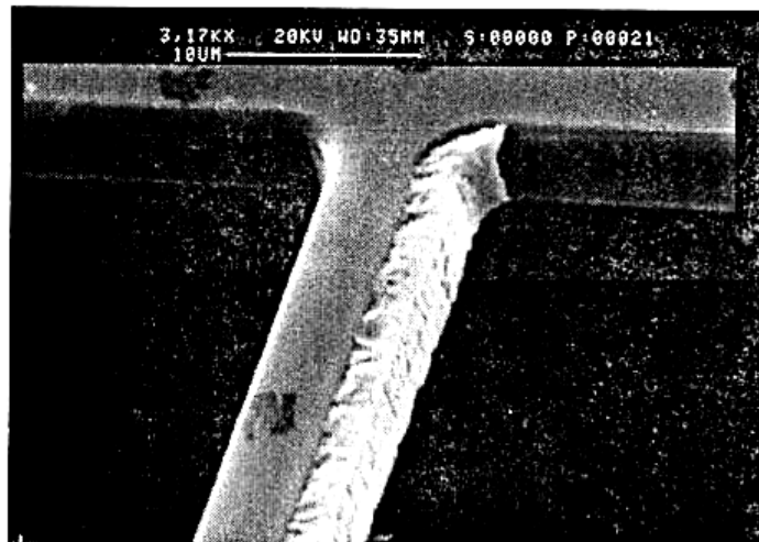
Figure 2.3: Thermal actuator made of silicon (w-5 \mu\text{m} ) and aluminum (w-2 \mu\text{m} ) (Barnes and Stephenson; 1994)
