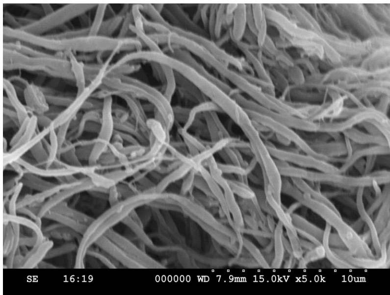
Figure 5.7 SEM observation of HDPE/PET composite.
