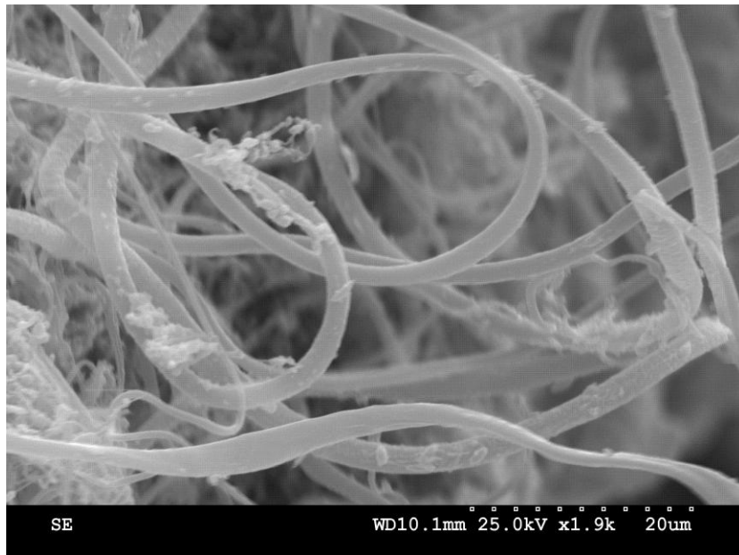
Figure 5.2 SEM picture of HDPE/PA6 composite.
