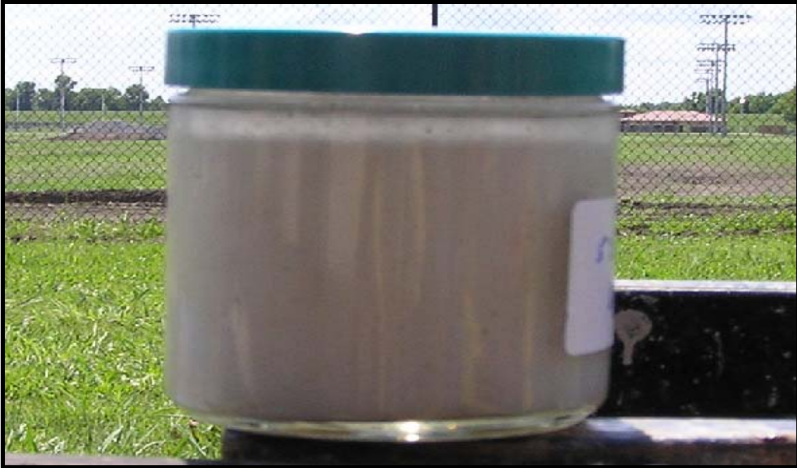
Figure 28 Sand Suspension in MF-55 (5% W/W) After Five Minutes
