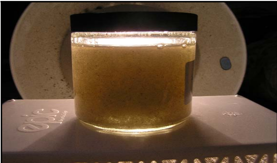
Figure 27 Sand Suspension in Xanthan (0.50% w/w) After 120 Minutes
