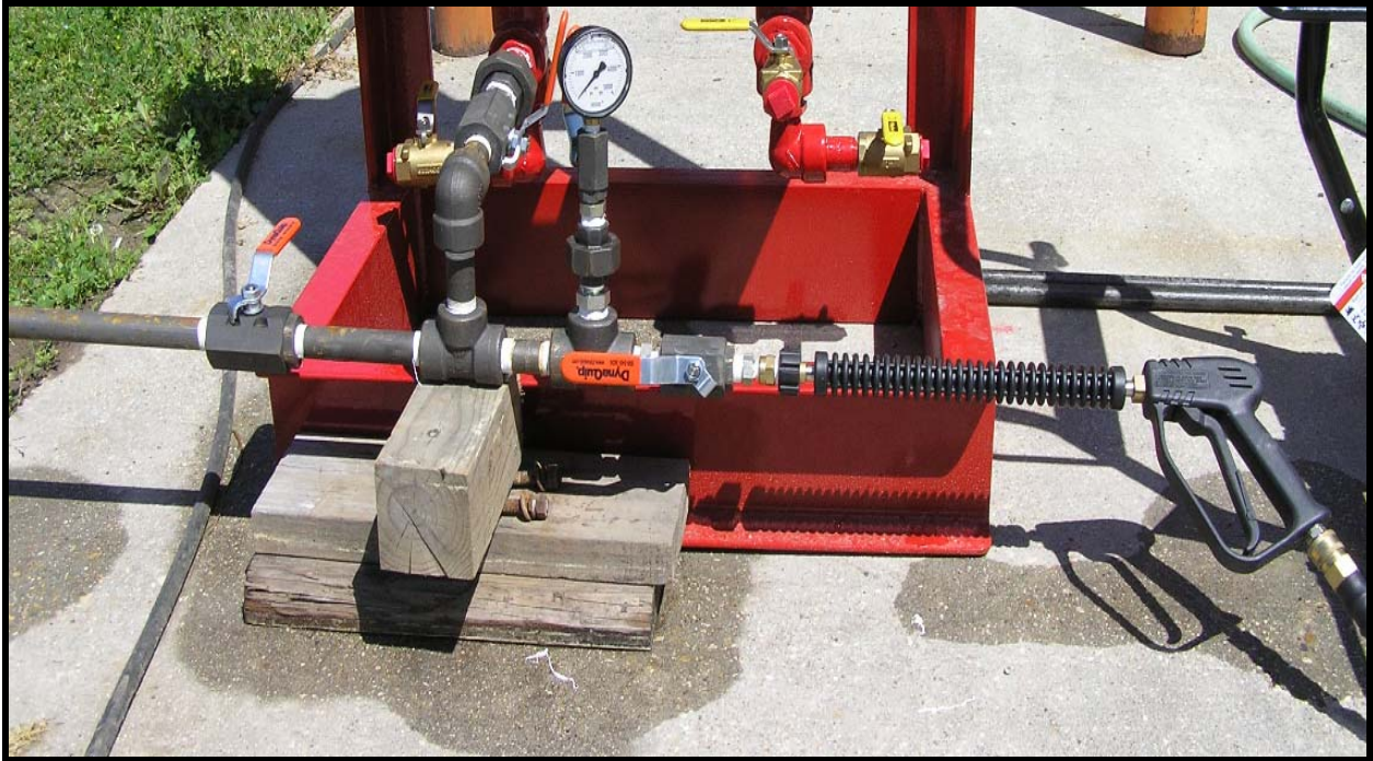
Figure 13 Experimental Apparatus for Pump Performance Curves
