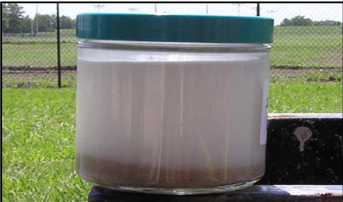
Figure 29 Sand Suspension in MF-55 (3% w/w) After Sixty Seconds
