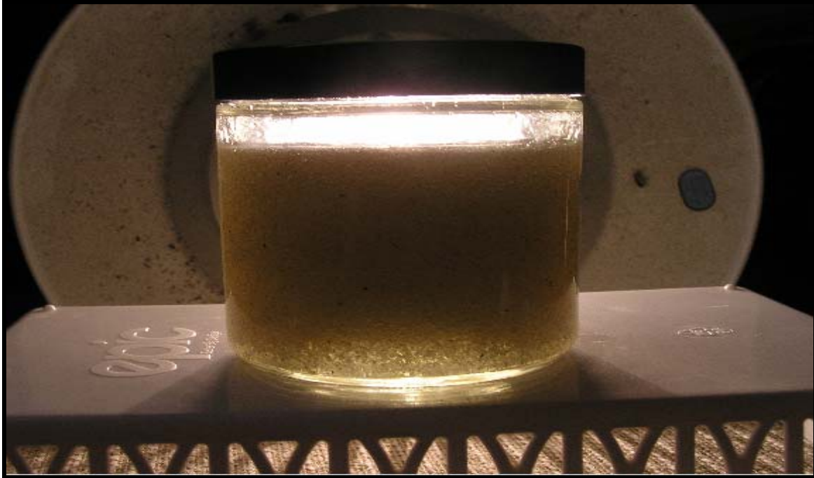
Figure 26 Sand Suspension in Xanthan (1% w/w) After One Week
