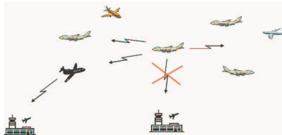
Figure 3.21. Use of 3DB for emergency communication in adverse conditions among airplanes as well as airplanes and ground stations
