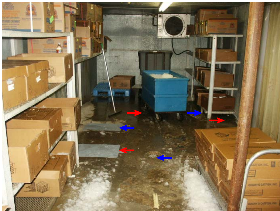
Picture 4. The sampling sites located by the walls and under the shelves in the walk-in cooler of plant B. Red arrows indicate copper-containing sites and blue arrows – their controls.
