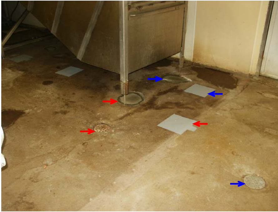
Picture 1. The sampling sites located by the boiling equipment in the receiving room of plant B. Red arrows indicate copper-containing sites and blue arrows – their controls.
