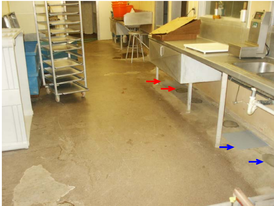
Picture 3. The sampling sites located under the weighing table in the packaging room of plant B. Red arrows indicate copper-containing sites and blue arrows – their controls.
