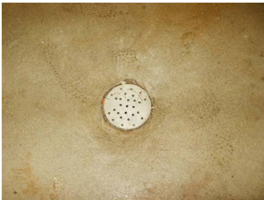
Picture 6. An original aluminum drain cover that served as a control.
