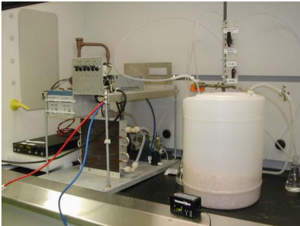
Figure 3.1. Set-up of the ozonation process.
