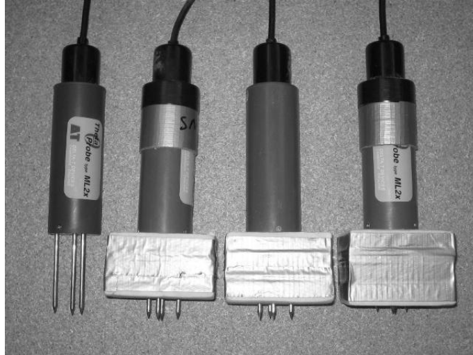
Figure 3.3: Delta-T Theta Probe inserted through dielectric foam blocks illustrating changes in sensor rod length from the manufacturer supplied 6.0 centimeters to lengths of 1.5, 1.0 and 0.5 centimeters.
