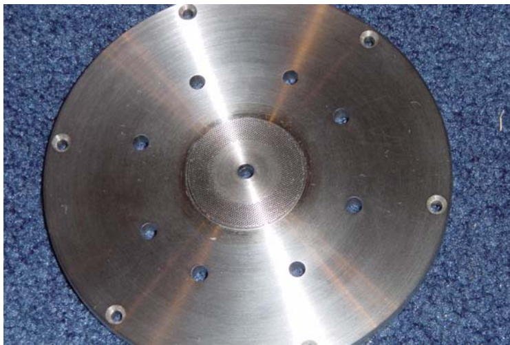
Figure 2-1: Mold Insert Used to Produce Silicone Mold
