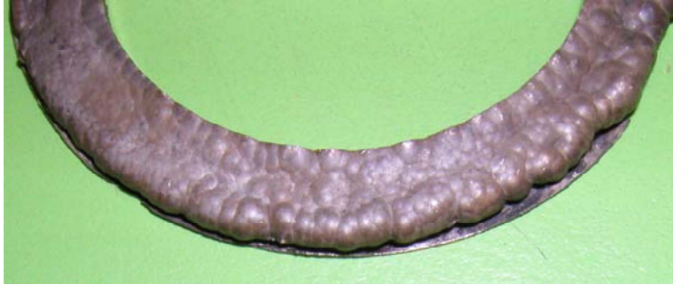
Figure 4-12: Typical Seal Top Surface after Electrodeposition
