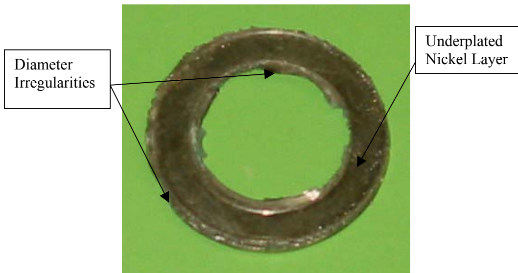
Figure 3-4: Underplated Nickel Formed During Electroplating
