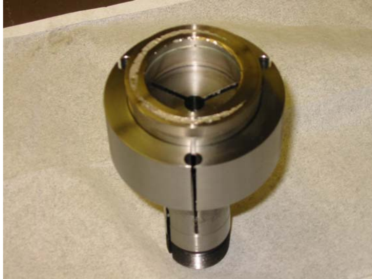
Figure 4-14: Seal Partially Machined and Held by Machined Collet
