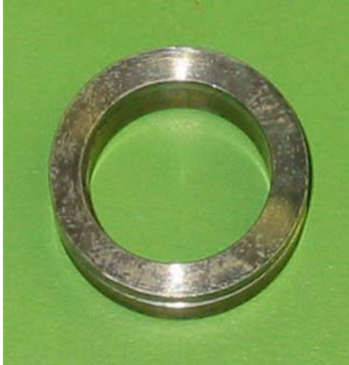
Figure 5-1: Top View of the Mechanical Seal's Nickel Surface
