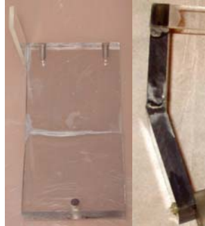
Figure 3-11: Plating Jig for the Activation, Wood's Strike, and Electroplating Processes
