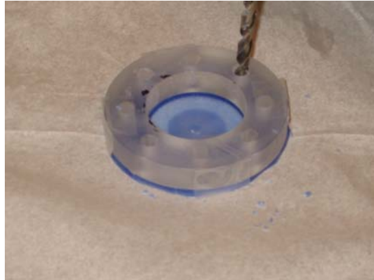
Figure 4-1: Drilling the Outer Wax Template Through Holes
