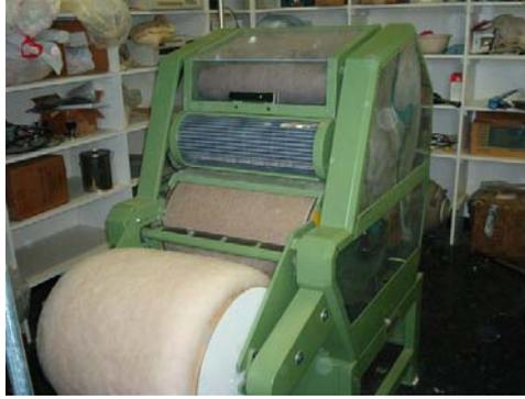
Figure 3-1 The LSU F015D Universal Laboratory Carding Machine
