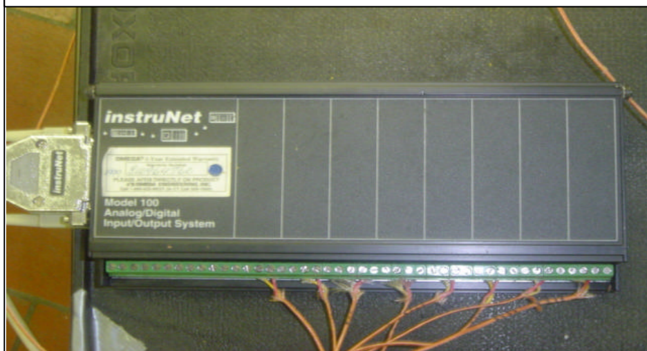
Figure 3.1 Instrunet interface terminal box
