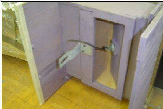
Figure 2.4 The by-pass gate
