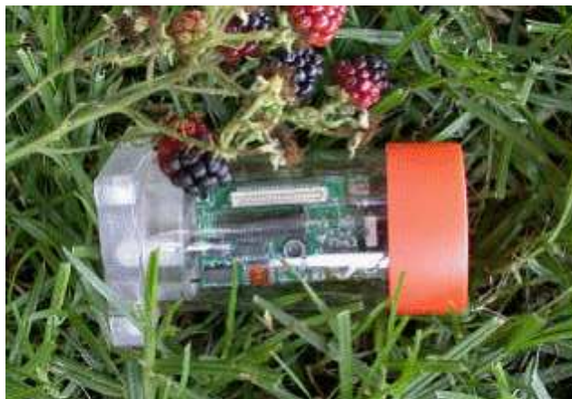
Figure 1.3: Enclosure to protect sensor nodes used to monitor the behavior of storm petrel.
