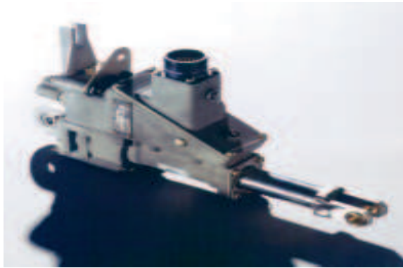
Figure A.1: Linear Actuator 658D100 for Rudder trim surface (Eaton Corporation)
