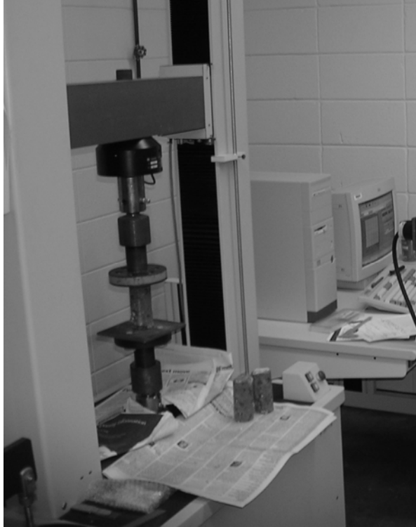
Figure 4: The Quotium Qtest load testing apparatus. This device was used to determine the compressive and flexural strength of concrete samples.
