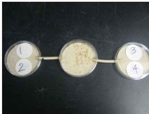
Pic4.2: Three Petri dish design with termites
