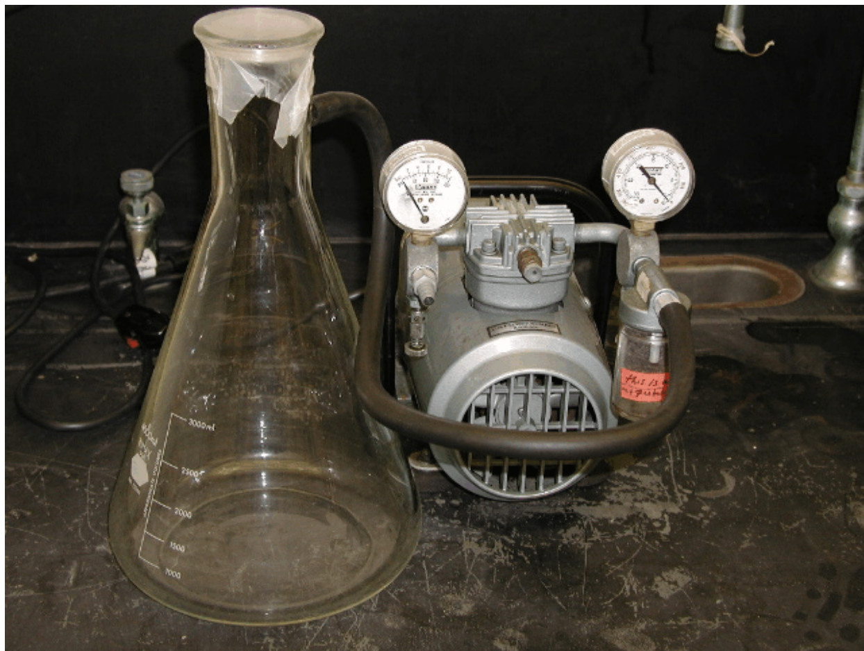
Photo 1: Pump setup for hydration under vacuum
