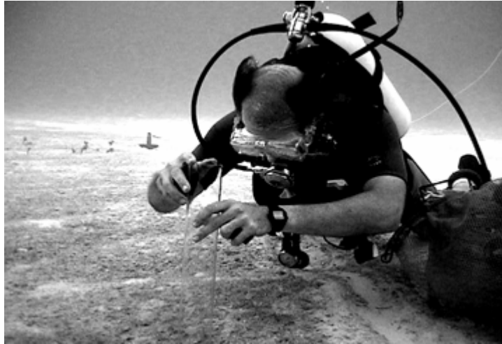
Figure 2.3. SCUBA diver (Kevin Briggs) prepares to insert a polycarbonate core tube, held between his hands, into ooid sediments south of Bimini, Bahamas. The core tube is 25-cm long, 6.1-cm in outside diameter (5.9-cm inside diameter), with a 1-mm wall thickness
