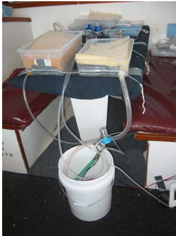
Figure 4: The foam-lined boxes and gill irrigation system used for the surgical procedure.
