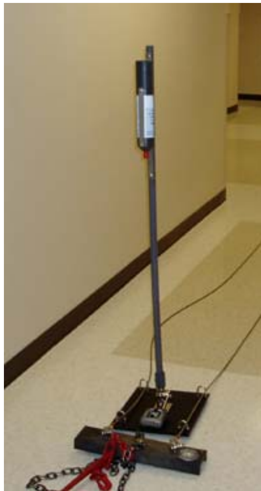
Figure 9: The receiver deployment system including a weighted sled that moved along two guide cables and PVC pipe to which the receiver was bolted, hydrophone end down.
