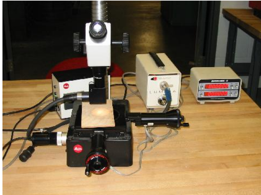
Figure 3- 9 Light section microscope used for wear measurements.
