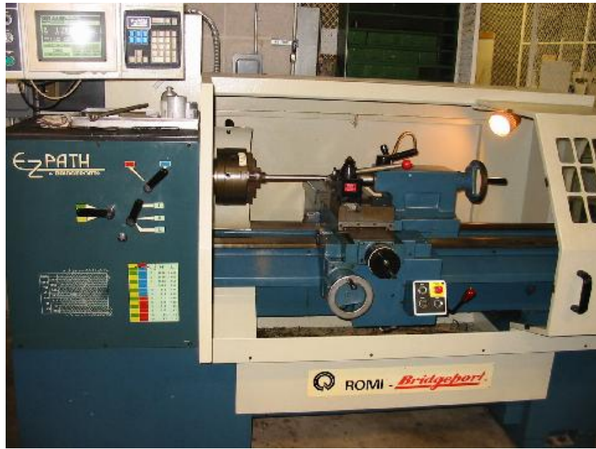
Figure 3- 1 Bridgeport EZ Path CNC lathe machine.
