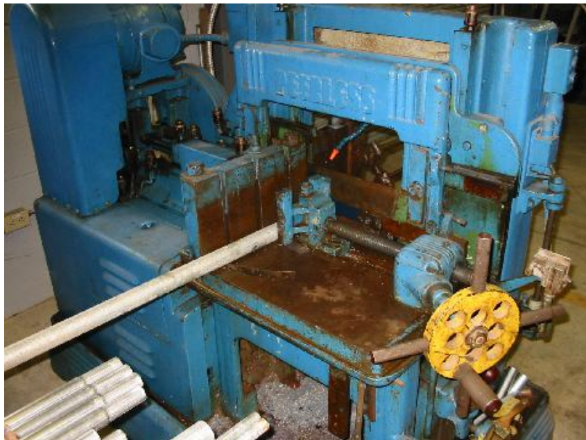
Figure 3- 6 Metal-cutter for cutting the work piece material.
