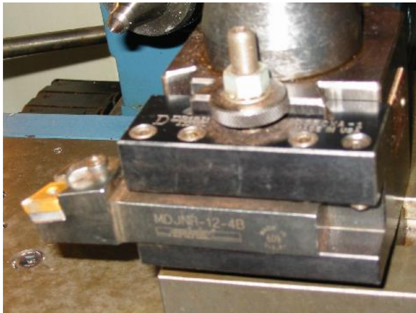
Figure 3- 2 The cutting tool and tool holder.
