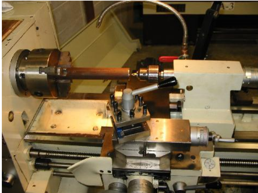
Figure 3- 7 Center drilling the work pieces.
