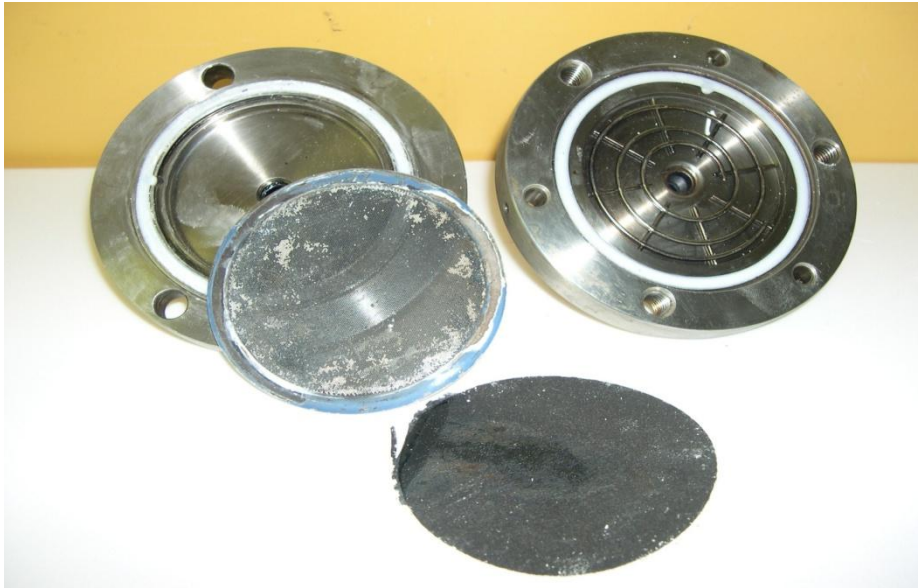
Photo B1: Filter Assembly showing filter paper with collected particulates after syngas sampling
