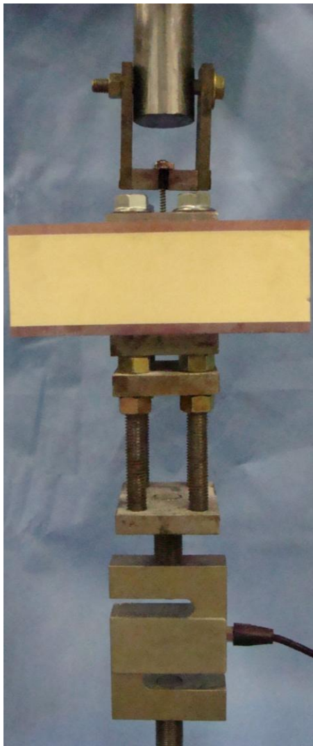
Figure 3.2. Photograph showing the AO pullout test construct in the MTS.
