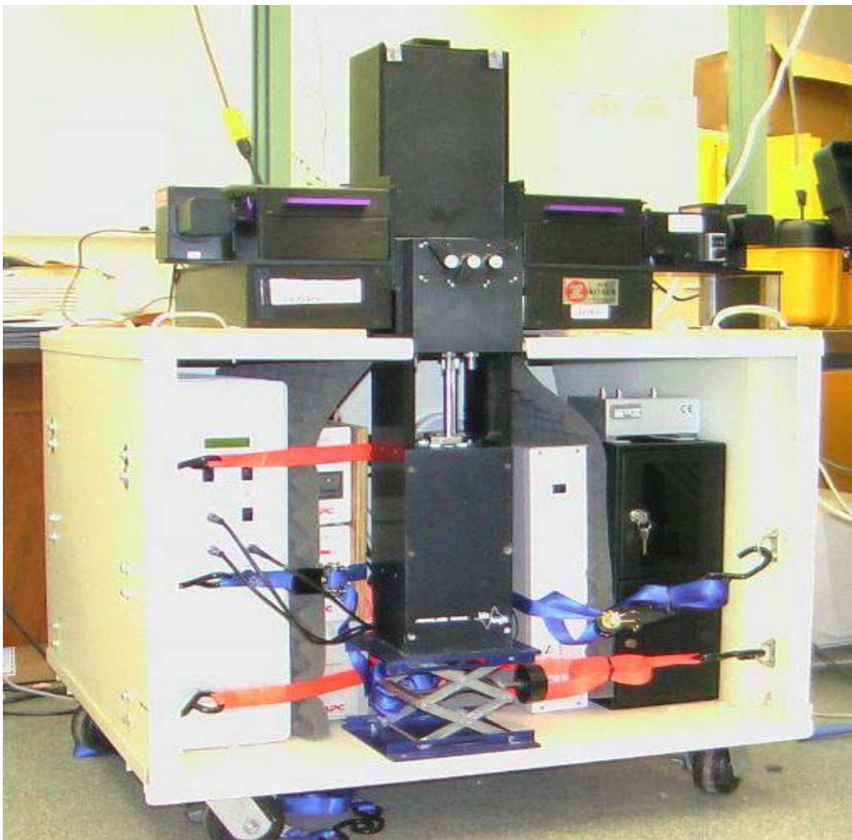
Figure 2.2: Fully assembled Cart #1. Visible in this representation are the fluorometer (horizontally oriented black box, sitting on top of the steel cart), the SFM-3 stopped flow (vertically oriented black box in the “center” of the cart), the data collection computer (right side, black), the PX01 photon counting electronics (white vertical tower, right side), the electronic controller for the SFM stepping motors (white vertical tower, left side), and the UPS units (next to controller, left side.) Also visible is grey padding, used as needed, and the cargo straps which served as the main support for most components. A lab-jack supporting the SFM-3 is also visible.
