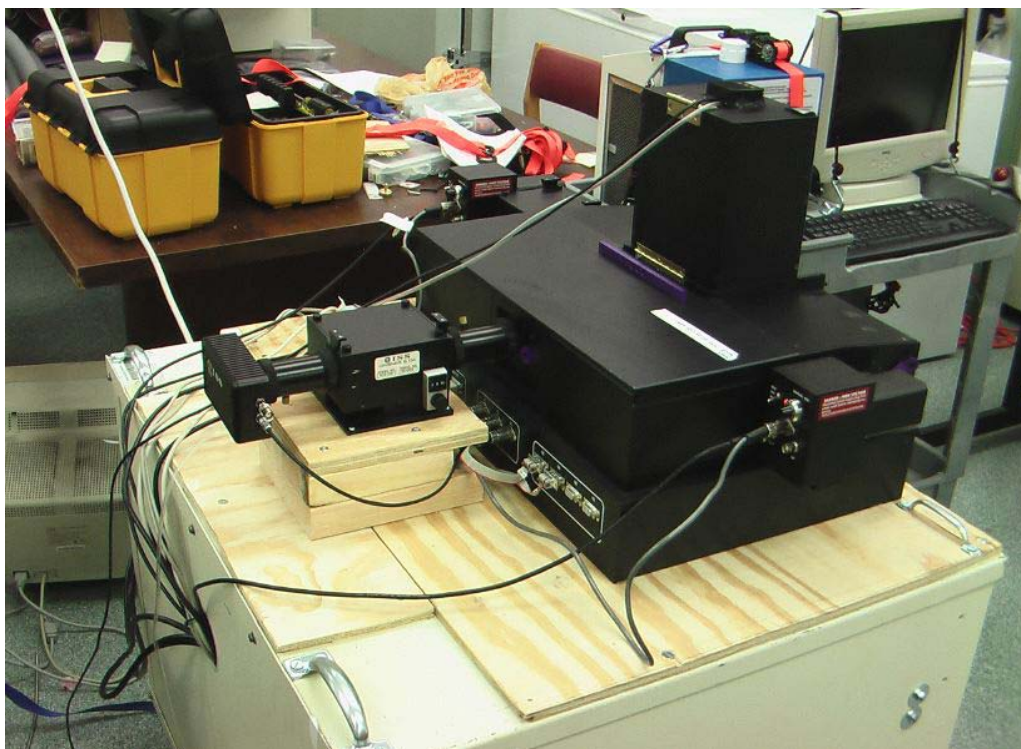
Figure 2.3: Rear view of Cart #1 in the foreground, with Cart #2 in the distance. Visible in this picture is the complex nature of the connections between the instruments and their associated components housed “inside” the cart. All connections to the component systems were run through the small port in the rear of the cart. Additionally, this view clearly illustrates the modular nature of the ISS Koala spectrofluorometer, as the photomultiplier tubes are visible on either side of the fluorometer housing with the monochromator and LED connected at the rear. Each of these components could be configured to allow any arrangement necessary.
