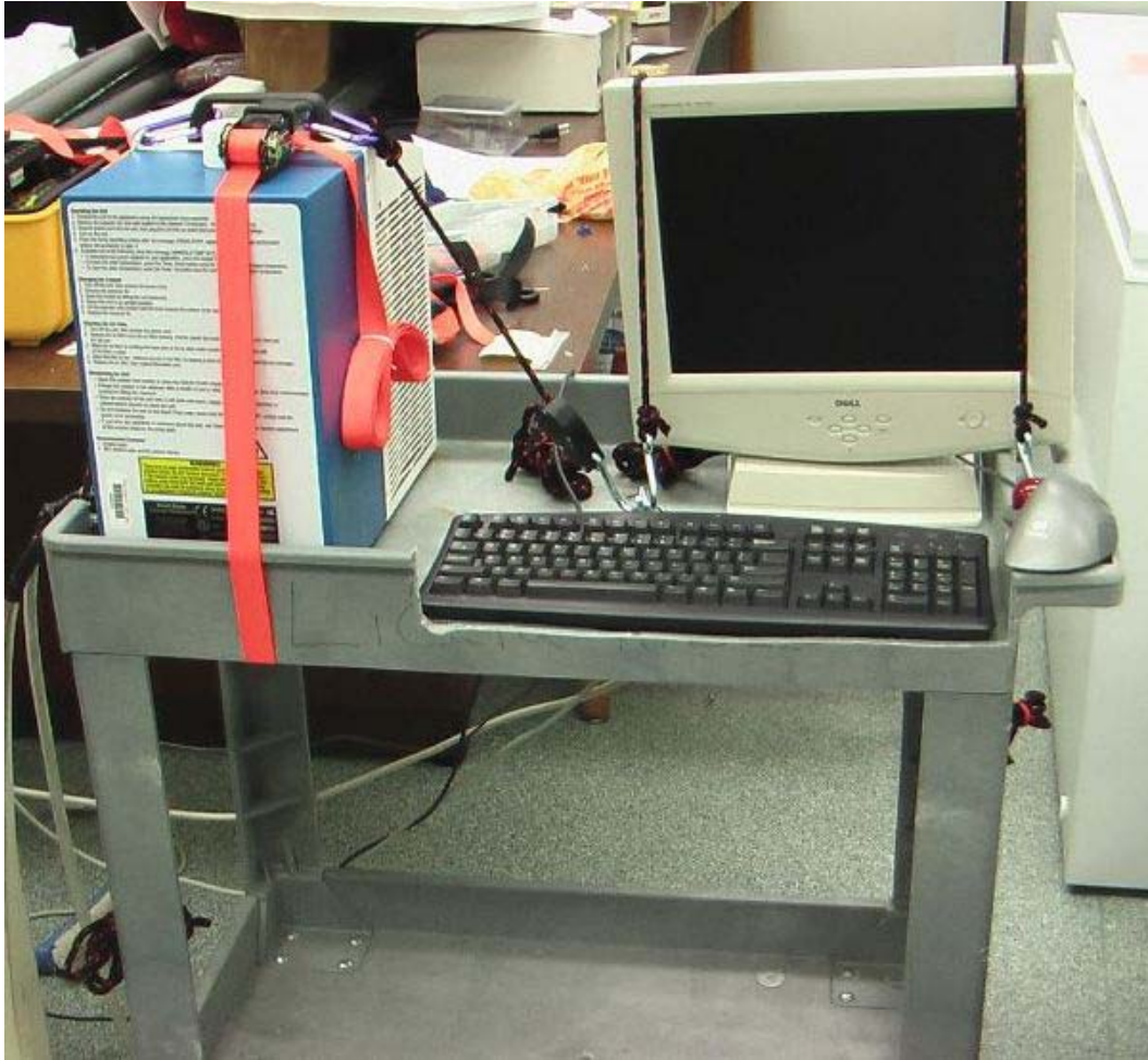
Figure 2.5: Fully assembled Cart #2. Visible in this picture are the Thermotek water-bath (left-side of the cart, attached with an orange cargo strap), the computer's monitor, keyboard, and track-ball mouse. Cargo straps and industrial grade Velcro were used to attach the various components.
