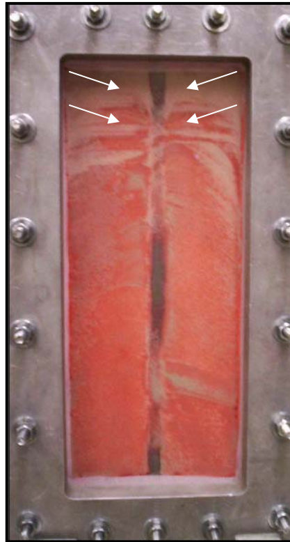
Figure 4.14: Gas Injection Profile into Water-Wet Fracture Simulation – 0.13 mm
