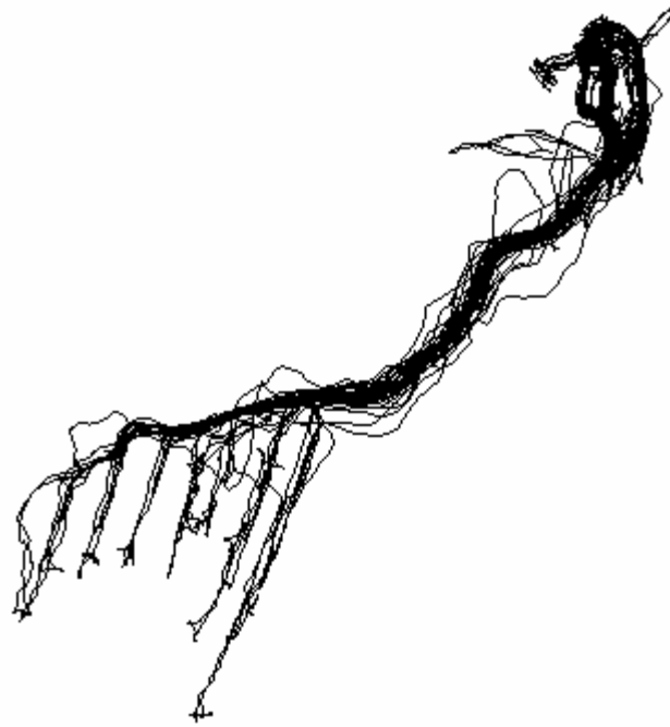
Figure 7. The GPS line file created by the skidder the afternoon of August 10, 2005. The GPS receiver was set to record a line on a 1 second time interval.
