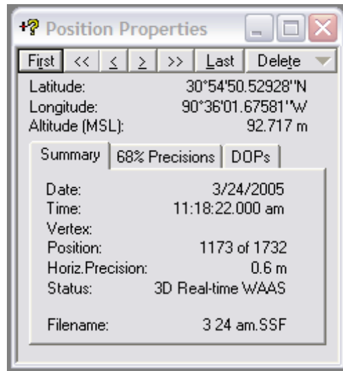
Figure 4. Position properties dialogue box shows the position, location and time data for each point is listed in a chart for quick reference.
