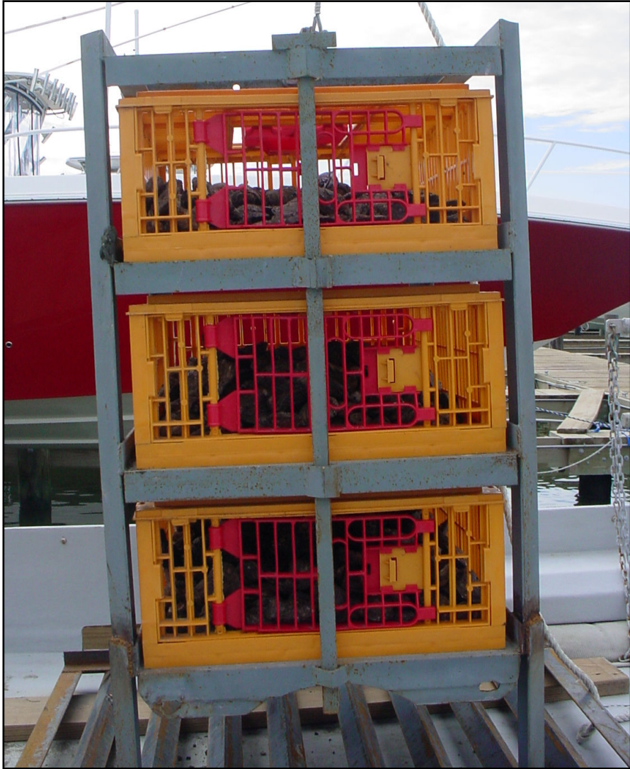
Figure 3.1 Photograph of oyster rack with oysters in chicken coops. The steel frame was 119x84x69 cm (42x33x27 in) and raised 30.5 cm (12 in) off the ground. The chicken coops contained a bushel of oysters and weighed approximately 100 lbs. each. The coops plus the frame weighed approximately 850 lbs.
