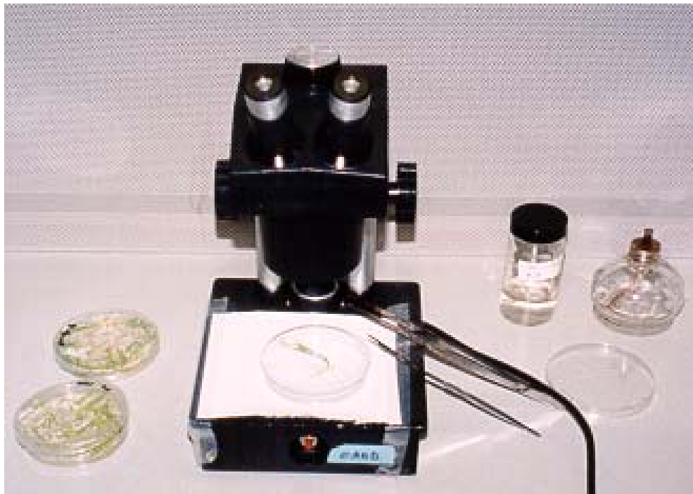
Figure 3.4. The apparatus needed for shoot apex isolation procedures performed entirely under a laminar hood.
