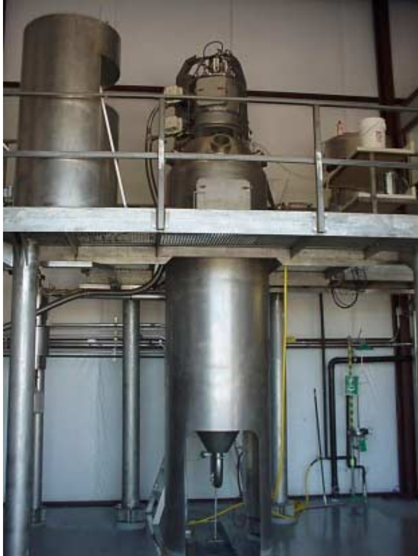
Figure 3. Photograph of pilot pulse combustion dryer at Pulse Combustion System's Research laboratory located in Payson, AZ.
