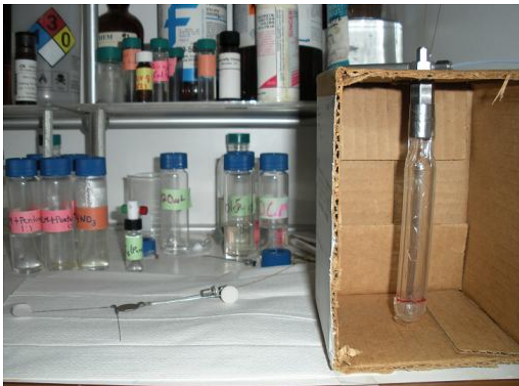
Figure 2-12: Apparatus for coating chips where coating solution in the test tube (reservoir) is passed through the nickel column with nitrogen flow
