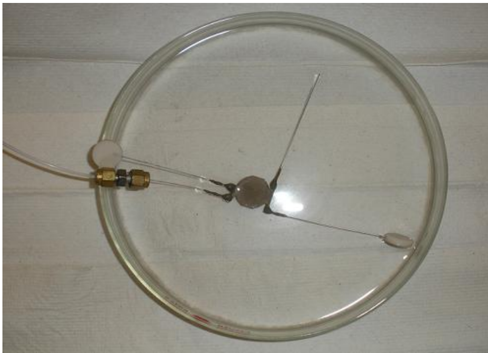
Figure 2-8: Testing chip for leaks with hydrogen flow in water
