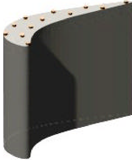
Figure 2.12. Blade tip with cylindrical pin fins.
