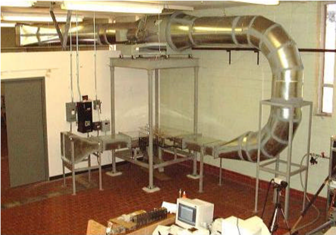
Figure 2.1. The overall layout of the facility and cascade test section.
