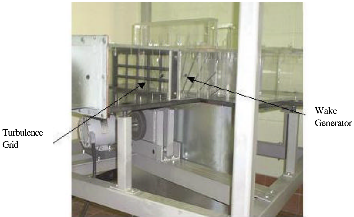
Figure 2.3. Turbulence Grid and Wake Generator as assembled in test cabinet.
