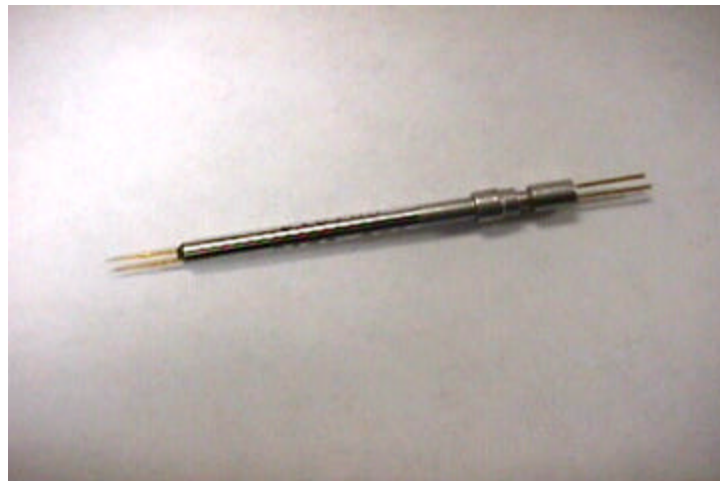
Figure 3.4(a) A single calibrated hot wire probe.
